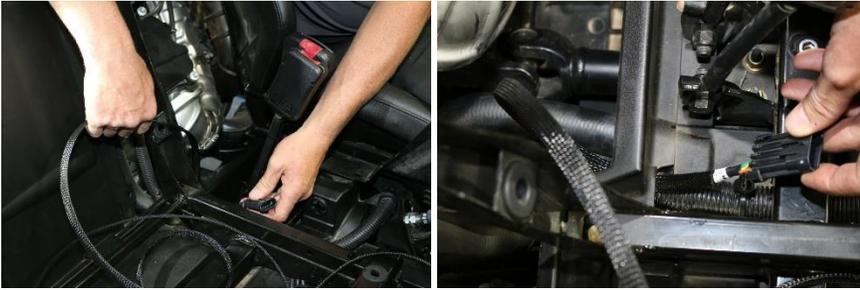
3. **Run the other ends**– of the rear harness with the Yellow wire to the driver's side panel, the one with the Green wire is run to the passenger side panel under the plastic rear panels that were removed where the cage goes into the plastics. Un-plug the factory harness and plug our harness in-line on both sides.
