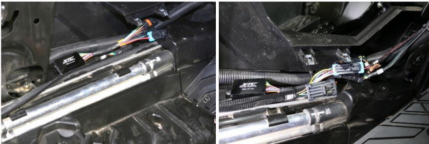
8. **Run power wire** – Plug the two pin Power Connector into the Control Module, run the other end up to the OEM busbar under the dash. Attach the ring terminal with the Red Wire to the left Keyed Power Post and the Ground to the Right Ground Post, do not connect to the center full time Power Post.
