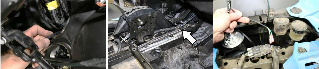
7. **Mount the Control Module**— Using the provided screw or cable tie mount the Control Module next to the main wire harness, Plug the front and rear harness in.
