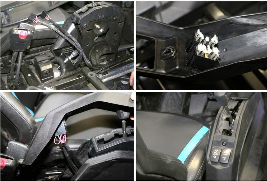
**Note: Dielectric Grease-** Just like the OEM uses on their switches, we recommend using Dielectric Grease on all switch terminals, this keeps the water out, thereby reducing corrosion and helps increase reliability! Open the grease and put on the switch terminals and the connector terminals on both the Turn and Horn switches, the more the better.
