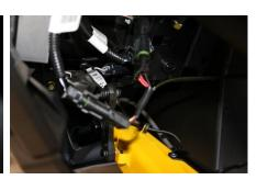
3. **Run the rear extension** – under the dash cover is the ECU and Busbar power posts. Un-plug the extension cable from the rear harness, un-roll and run the female down the fire wall behind the ECU to the center panel, follow through the center to the previously installed rear harness and plug in.
