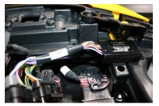
6. **Install Front Harness** - Un-roll the front harness, plug into the control module, run the cables with the yellow and green wires through the frame tube leading to the top of the radiator. Also remove the Headlight rear covers to run the wires.
