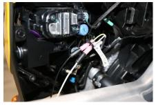
Run the green and white wires to the right/passenger side LED, run the yellow and white wires to the left/driver's side LED. **NOTE:** Black wire is positive and goes to Green and Yellow, white is ground, they will not work if reversed. Secure the Harness using the provided cable ties.
