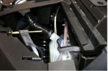
10. **Install Horn** – Remove the screw shown below and use the removed screw to mount the horn. Attach violet and black wire from front harness to horn terminals, polarity does not matter.
