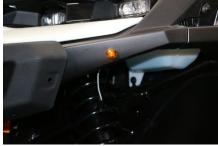
12. Attach Front Harness to lights - The Green and white wire go to the right/passenger side LED, attach the Green to the Black and the White to the White, the Yellow and white wire go to the Left/Driver side LED, attach the yellow to the Black and the white to the White. NOTE: Black wire is positive and goes to the green and yellow wire, they will not work if reversed. White is ground. Pull any excess wire back under the dash and secure the Harness using the provided cable ties.
