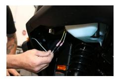
**13. Run power wire** – Plug the power cable into the ATS Control Module. Unplug the accessory power harness from the white holder shown below in the dash, plug the ATS power cord into that cord. The White cap is not used.
