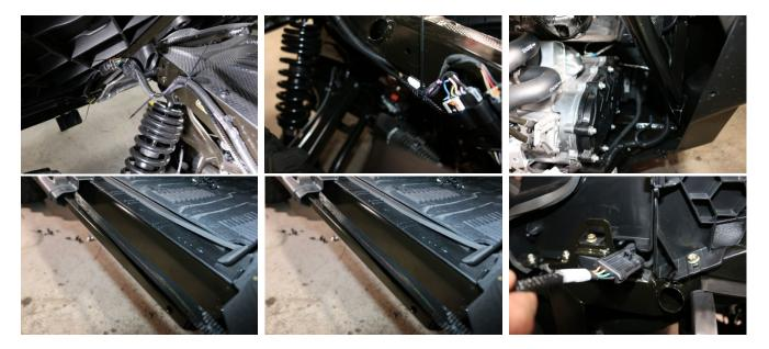
4. **Remove the A-Pillar covers** – To gain access to the dash cover screws the A-Piller cover need to be removed. If a windshield is installed, only remove one strut at a time, then the plastic and reinstall the strut, then remove the other side.
