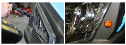
5. **Install Horn** – In the front near the passenger headlight, remove the bolt for the front support bracket and install the horn as shown.
