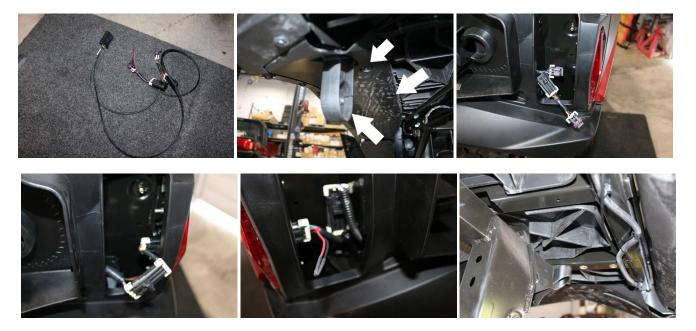
**3.** Run the Rear Extension cable – Un-roll the long harness, plug the extension into the just installed rear harness, take the other male end and run it along the factory harness to the rear firewall.
