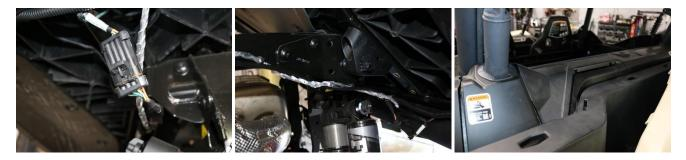
Remove the cover on top of the rear firewall where the roll cage goes in. Run the cable up the firewall behind the air intake tubes, follow the factory harness through the firewall and down past the ECU and battery.
