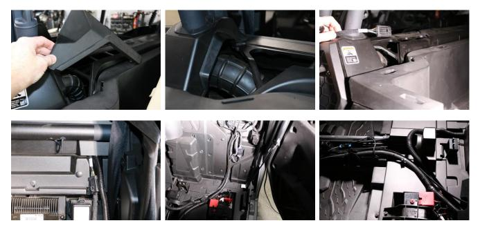
Follow the factory wire harness up to the front of the center tunnel next to the accelerator pedal.
