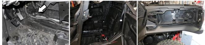
2. Install the Rear Harness – The rear harness plugs in-line with each taillight. The taillight plug is accessed by removing the side cover off the dump bed. Remove the side marker reflector and two Torx screws. The harness will be installed next to the factory harness, take the plugs with the yellow wire and run through the bottom of the dump bed to the left/driver's
