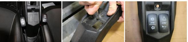
9. Install Switch Harness – Plug the large switch connector into the Control Module and run the Switch Connectors to the switches. Apply grease to the Switch Terminals and plug switches into connectors and re-install plastic cover.
